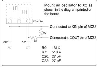
Figure 5 Connection diagram of X2 socket
